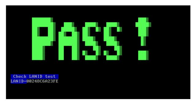
This chapter shows how to use the Diagnostics to test the MAC address of the Ethernet controller.
